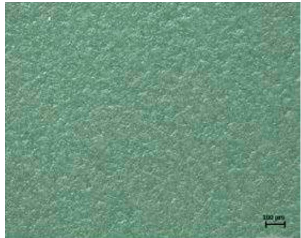
Figure 10. View of the surface of the topcoat of the SP2 masking system
