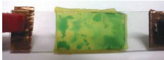
Fig. 2. Electrochromic cells change their color with the voltage applied
