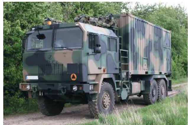
Fig. 2. A military vehicle coated with a camouflage paint scheme utilizing certified Polish-manufactured paints (photograph by the author)
