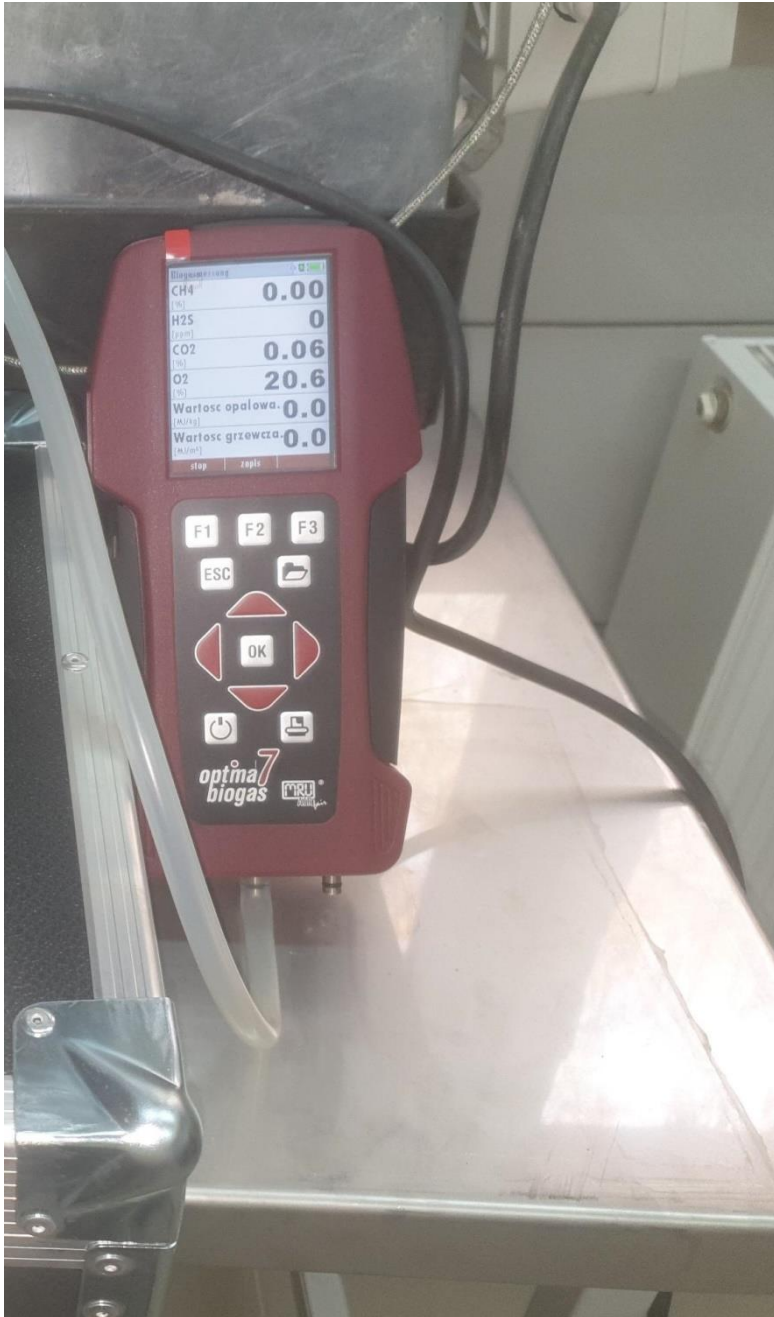
Ryc. 4.13. Analizator biogazu Optima 7 Biogaz MRU
